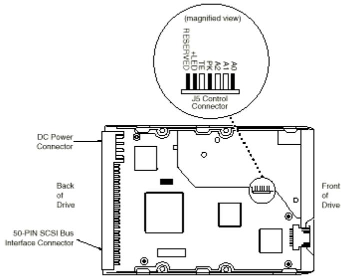
**Figure 3-3** Jumper Locations on the Drive PCB
